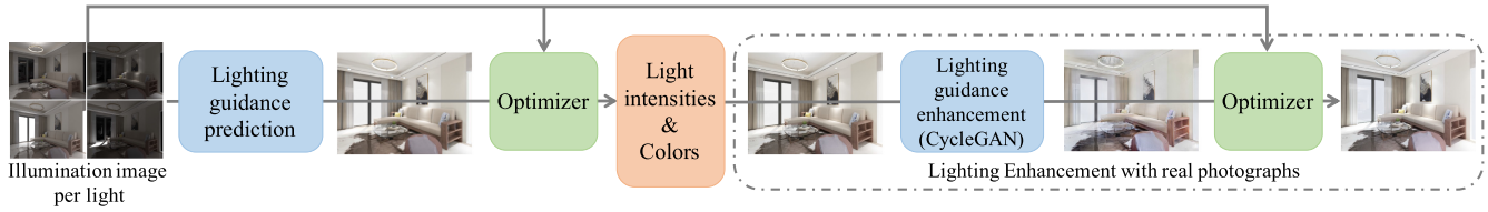
Fig. 7. Light emission optimization pipeline. Our light emission optimization pipeline consists of two steps, guidance image prediction and optimization, as shown in the blue and green blocks, respectively. Our pipeline can also utilize real-world photographs to enhance our lighting effects with CycleGAN.
