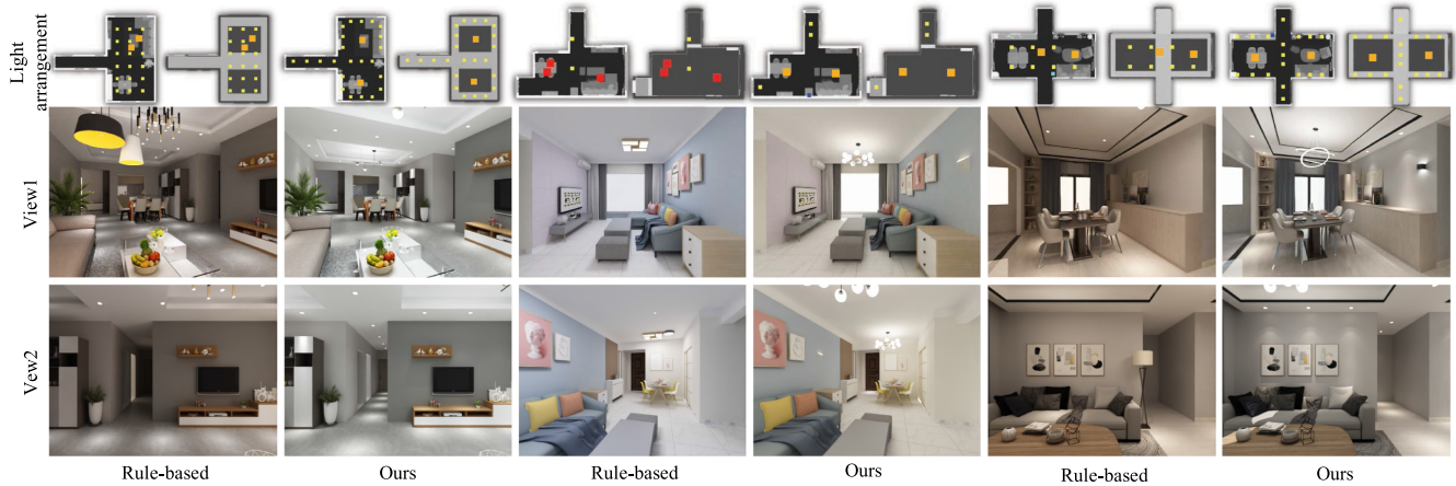
Fig. 10. Visual comparisons of the rule-based method and our method. The top row shows the visualizations of the light arrangements from top-down and bottom-up views. It is seen that our method can generate light layouts that better fit the room structure and furniture arrangement. Sufficient lighting for the whole room is achieved in our method, while the rule-based baseline often fails to place downlights in the corridor. Inappropriate arrangements of key lights (e.g., not suitable for the ceiling pattern, no or multiple key lights in one space) also appeared in the results of the rule-based baseline.
